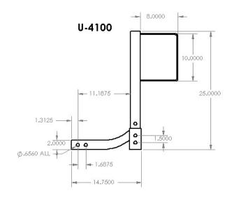
The Hornet U-4100 S is a Fold Down hitch designed for autos, trucks, and RV's where you require a heavy duty mount and features the convenience of easy access to your tailgate or rear compartment. This hitch is rated to carry a spare up to 100 lbs.
