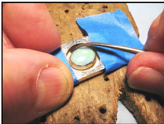
Painter's tape applied to protect the surface.
