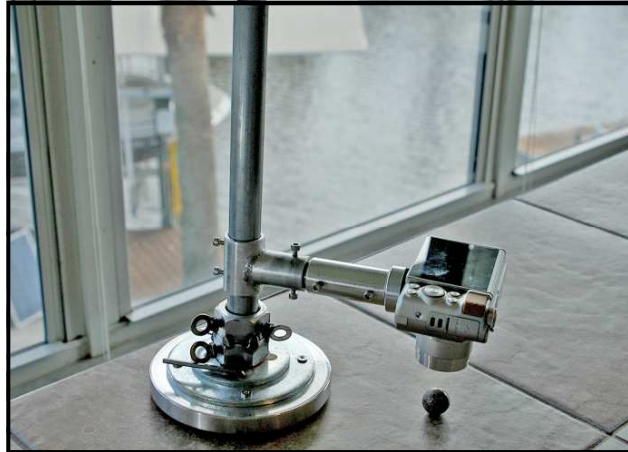
The copy stand with the camera focused on a dinosaur bone sphere.
