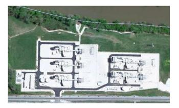
Bluegrass Power Generation - 624 MW, outside Louisville, Kentucky Greenfield site selection, Development, Permitting, Financing, Tax Abatement Package, EPC and Construction to Operations Three Siemens 501F turbines in simple cycle into LG&E 345kv line, in ECAR
