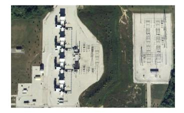
Rockwood Energy Center - 1,068 MW 2x1 Combined Cycle plant with 345kv transmission on site and gas supply in 7 miles Columbus, Texas west of Houston. Greenfield Site Selection, Development, Permitting, Gas & Power Transmission
