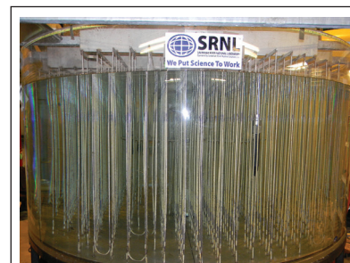
A TOUCH OF REALISM A scale model of the cooling coils found in the waste storage tanks was placed in the experimental tanks.
