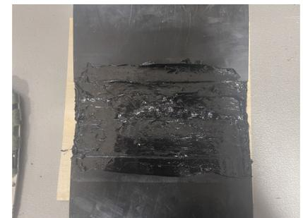
Once the splice is fully sealed, or the fastener is fully covered, leave to cure for the recommended times before restarting belt operation. (see back of brochure)
