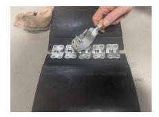
When covering belt fasteners, we recommend that the belt is skived back approx. 1 inch on either side and the fasteners are countersunk to leave them flush with the top cover.
