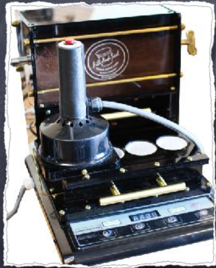
4 Cup Manual unit: Turn key to load coffee into cups
