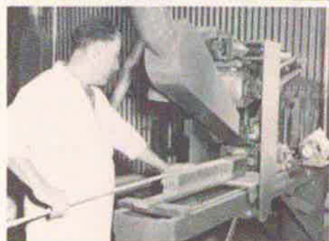
A Handle Contour—with this machine each handle is sanded to exactness that could not be obtained by any other process. Weight saving core laminations are sanded within .002 of an inch on this machine. Wing manufactures all of their laminations from hard northern straight grain maple cut in their own plant. No maple veneer is used in a Wing bow.
