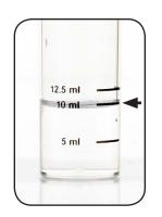
3 Add OP Titrant (AD1596) one drop at a time while swirling. Count the number of drops until the sample color changes from green to purple. A gray intermediate color may develop. Keep titrating to the purple endpoint.
