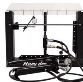
Determination of deflections with center and off center, normal and vector loading; photoelastic observation of stress patterns and values with a polariscope.
