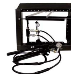
Determination of structural characteristics, derivation of theory, observation of stress patterns, evaluation of stresses. For use with 4 photoelastic diagonals - arranged with 2 short and 2 long photoelastic diagonals to demonstrate redundancy and stress patterns with polariscope.
