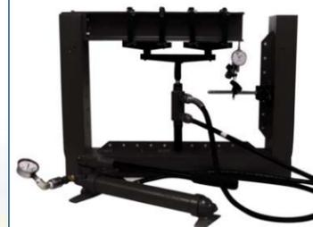
Determination of deflections and stresses of point or distributed loads in cantilevered beam.
