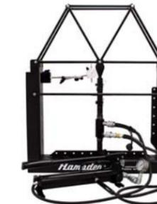
Determination of deflections at all critical points in model, failure predictions based on materials properties. Includes clevis and attachments arranged for center loading of bottom middle spacer.
