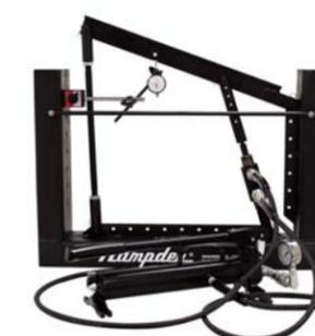
Determination of vector effects, stress distribution, deflections, composite force effects. Includes clevis and attachments arranged with anchored end, and with capability for applying load near center of truss.
