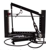
Determination of vector effects, stress distribution, deflections, composite force effects. Includes clevis and attachments arranged with anchored end, and with capability for applying load near center of truss.
