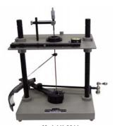
Model H-6311 Torsion Test Demonstrator
