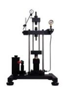
Model H-6310 Hydraulic Tension Testing Machine
