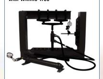
Determination of deflections and stresses of point or distributed loads in cantilevered beam.
