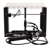
Determination of deflections with center and off center, normal and vector loading; photoelastic observation of stress patterns and values with a polariscope.
