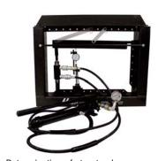
Determination of structural characteristics, derivation of theory, observation of stress patterns, evaluation of stresses. For use with 4 photoelastic diagonals - arranged with 2 short and 2 long photoelastic diagonals to demonstrate redundancy and stress patterns with polariscope.
