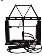
Determination of effects of loading statically indeterminate structure designs. Includes clevis and attachments arranged for center loading of bottom middle spacer.
