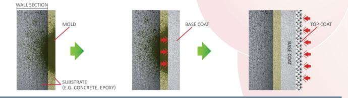
Quite often, residual moisture, mold, and mildew of building surfaces are only partially visible. Moisture, spores and fungal biomass are in deeper layers of the substrates. (e.g. concrete, epoxy) After mechanically cleaning the substrate *Bioni System* base coat can be applied directly on the mold affected substrate.
