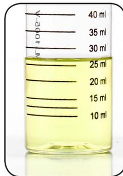
**4 Add Chloride Titrant** (SN3410) one drop at a time while swirling. Count the number of drops until the sample color changes from yellow to red. The first color change is the endpoint.
