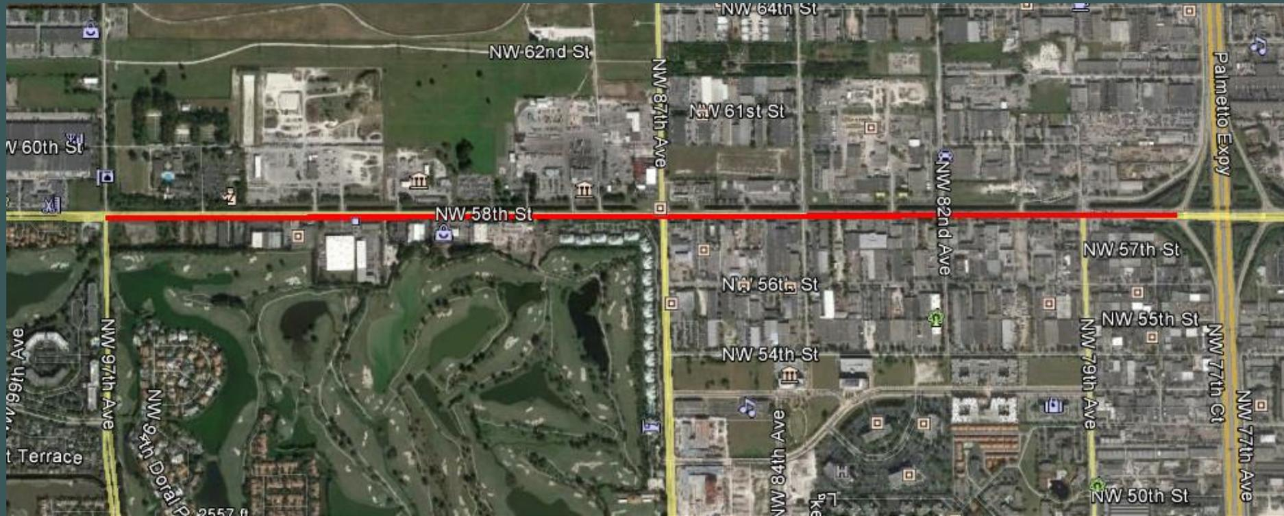
**SCOPE:** The project consists of master planning, public involvement, and preparation of complete construction plans to reconstruct the existing road to a 4-lanes roadway with continuous center turning lane, bike lanes, sidewalks, curb & gutters, storm water drainage system, pavement markings and signage, upgraded traffic signalization and roadway lighting.
