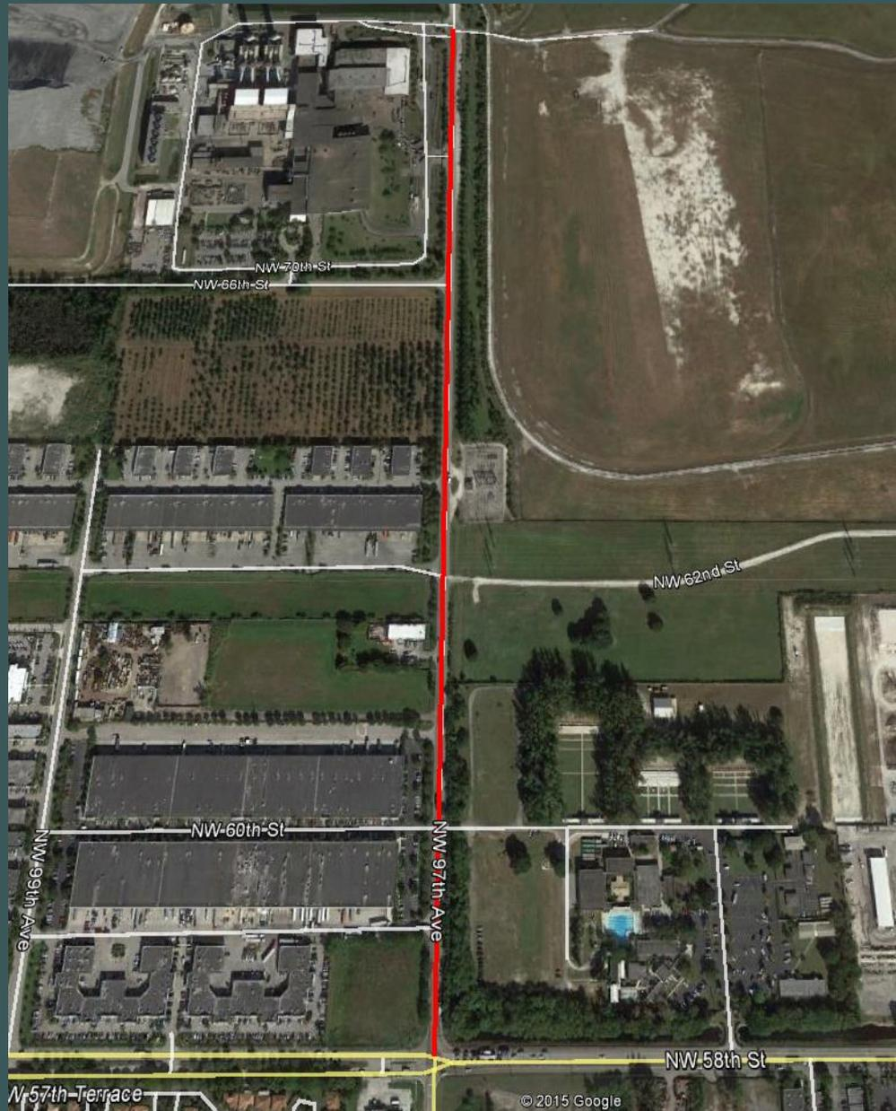
**SCOPE:** The project includes master planning, public involvement meetings, and preparation of the complete construction plans to provide roadway improvements to NW 97 Ave which may include, widening to a 4 lane divided road, sidewalks, curb and gutters, bike lanes, storm drainage system, pavement markings and signage, signalization, lighting, and landscaping.
