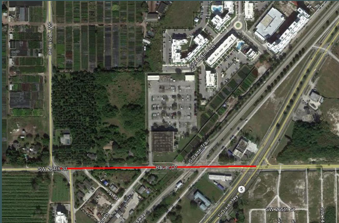
**SCOPE:** The project consists of widening the existing roadway to a 2 lane divided roadway with center turn lane, bike lanes, on street parking, sidewalks, curb and gutter, storm drainage system, signalization, pavement markings, signage, and lighting.
