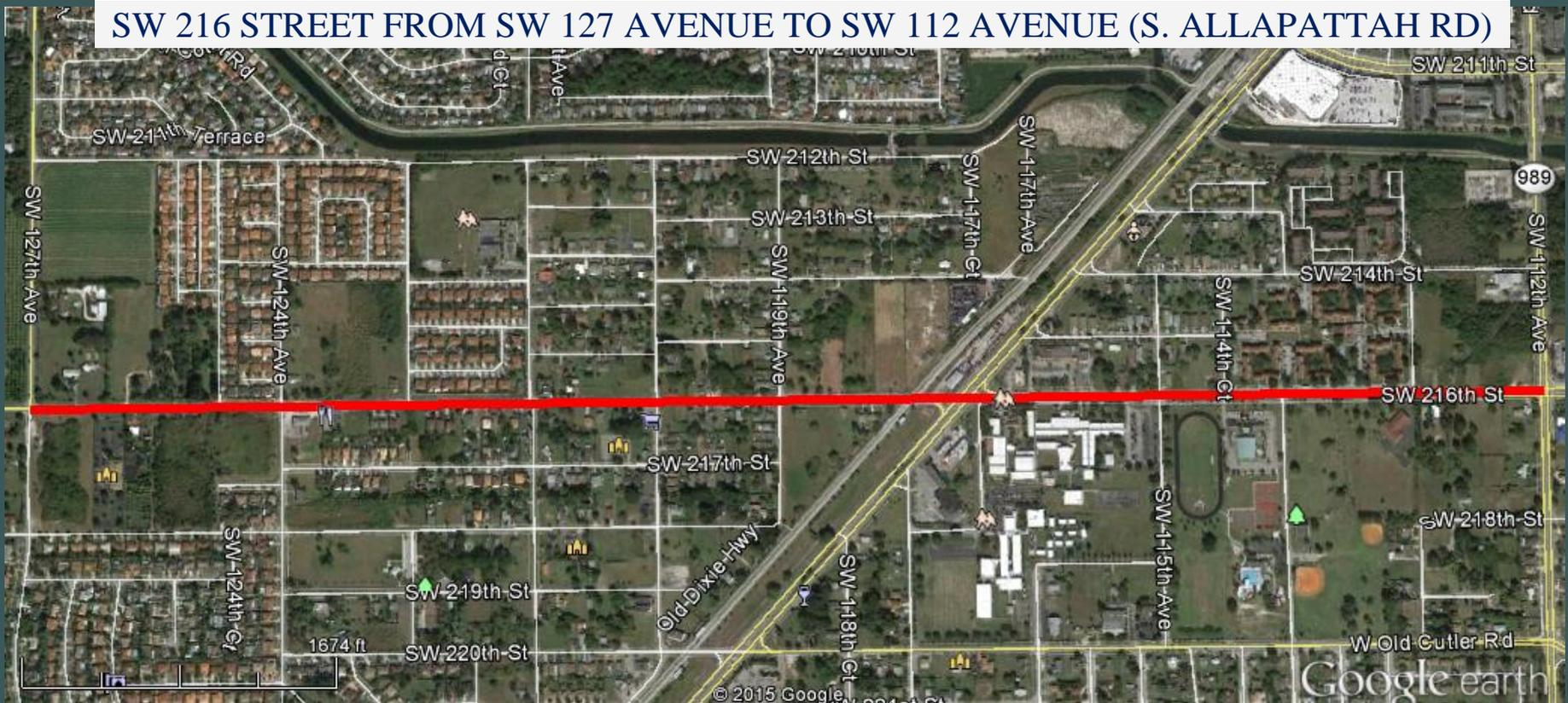
**SCOPE:** The project consists of widening the existing roadway to 2 lane divided highway with a raised landscaped median, bike lanes, on-street parking, sidewalks, curb and gutter, new storm drainage system, signalization, pavement markings, signage, and lighting.
