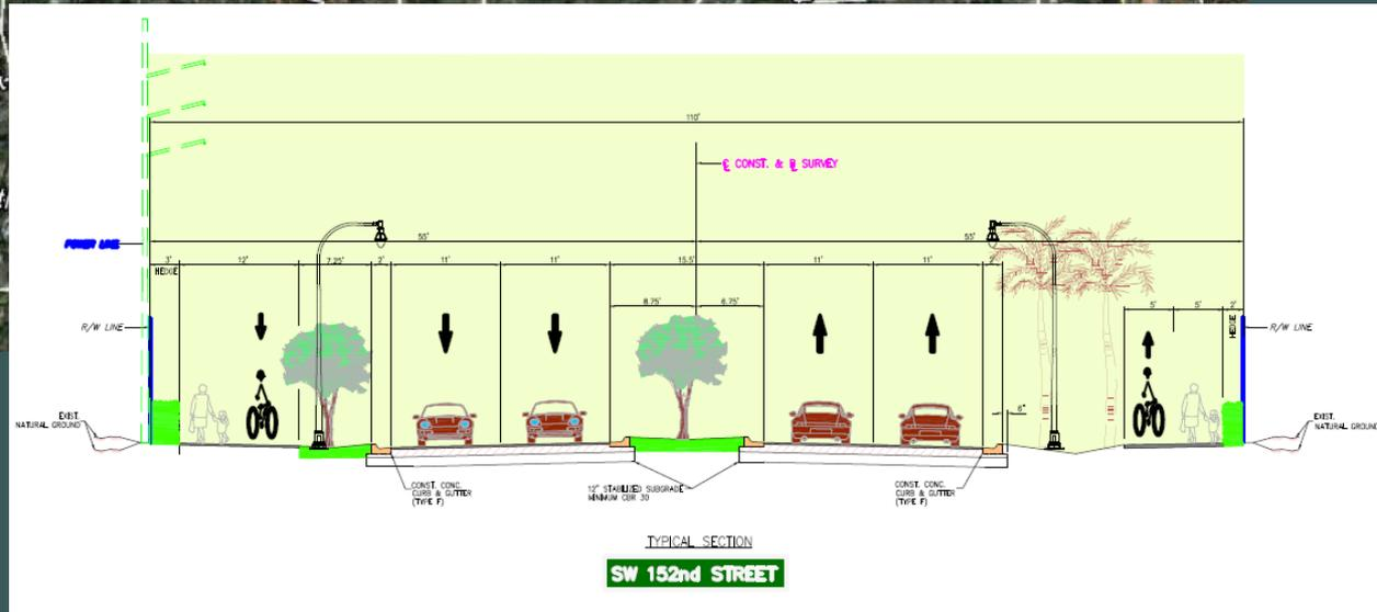
**SCOPE:** The project consists of widening the existing roadway from 2 to 4 lanes with a median, Shared use paths, curb and gutter, continuous storm drainage system, landscaping, signalization, pavement markings and signage, and decorative lighting.
