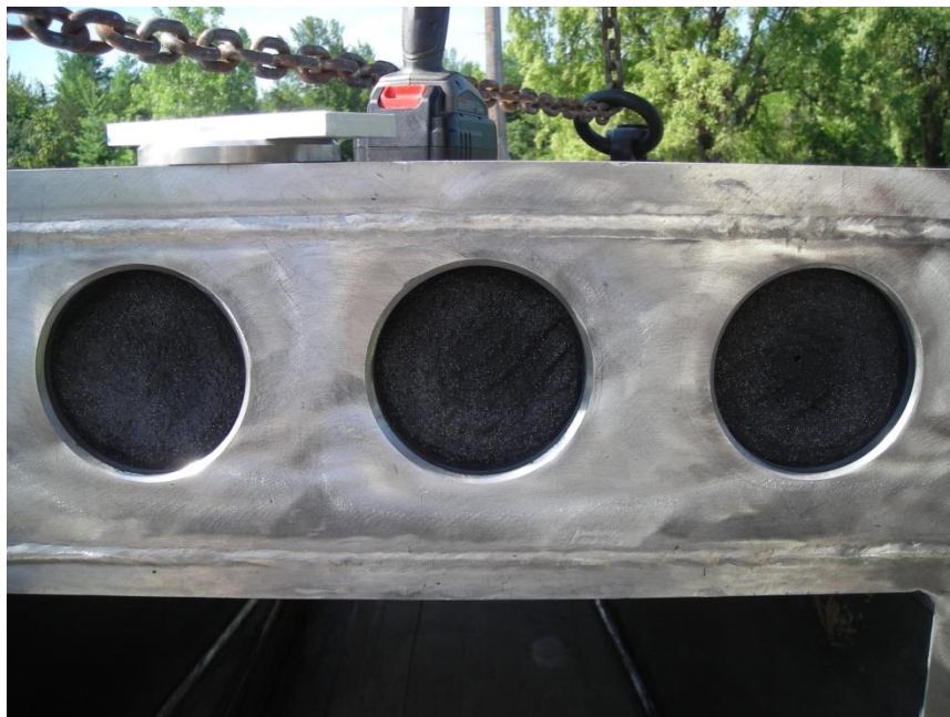
Figure 4. Cryostat plug filled with MS1-a mixture
