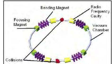
In an accelerator ring, focusing magnets and bending magnets guide the beam of particles. High frequency microwave cavities accelerate the beams as they pass through.
