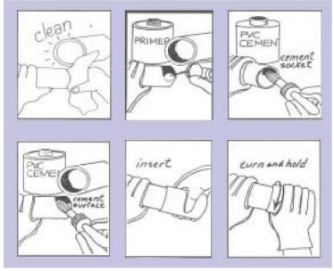
Select the proper cement for whichever material you are installing and the use conditions (e.g., pipe size and temperature). Check for the material designation (e.g., ABS or PVC), the ASTM number, and for a certifying laboratory seal or mark on the can.
