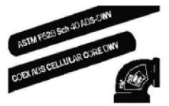
None of the other DWV pipes are pressure rated.
