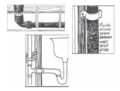
Codes require transition from one material to another only through use of approved adapters or joints. Your supplier should have a selection of plastic adapters. In addition, some codes approve clamped, flexible connectors or hubless couplings as adapters between cast iron and plastic piping.
