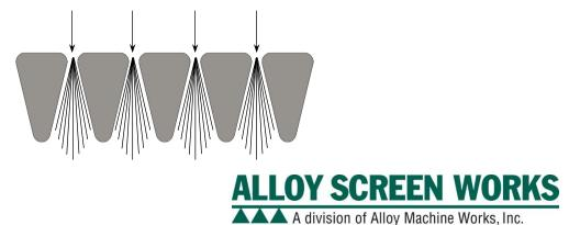
**The Strength** of these screens is due to the all-welded construction of the wrap wire being welded to the rods at each point of contact. Heavy rod configurations help to distribute the driving forces evenly throughout the screen without sacrificing open area.
