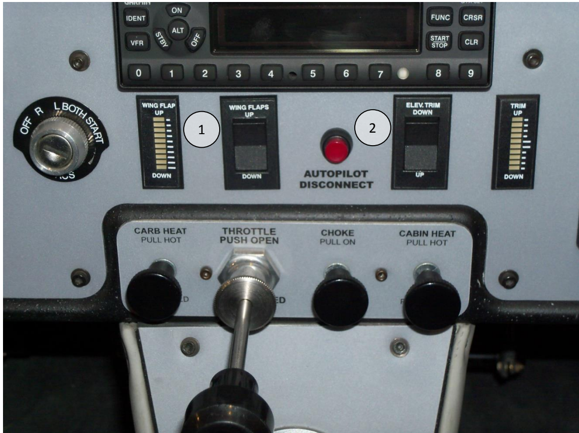
Figure S11-4: Elevator Trim and Flap Switches with LED Indicators
