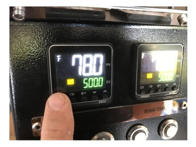
The first menu setting is the one you need to change the thermocouple type. Regardless of the number it shows switch to this setting:
