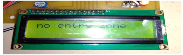
Fig.11. No Entry Zone indication
