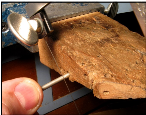
Cutting a small tube to length with a saw.
