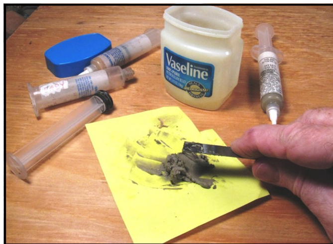
Mixing paste solder with Vaseline.
