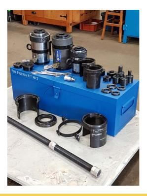
HEMS Pin Puller Kit, includes both a 30ton and 50ton jack, suitable for various applications.
