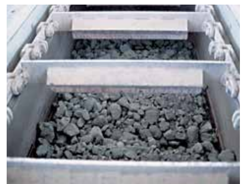
View into Chain Conveyor
