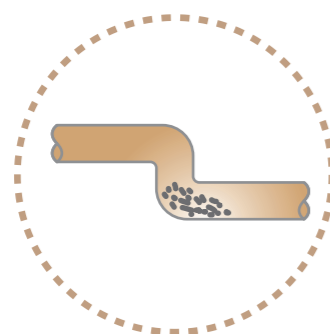
Piping used with R22 refrigerant has mineral oil attached to its surface.
