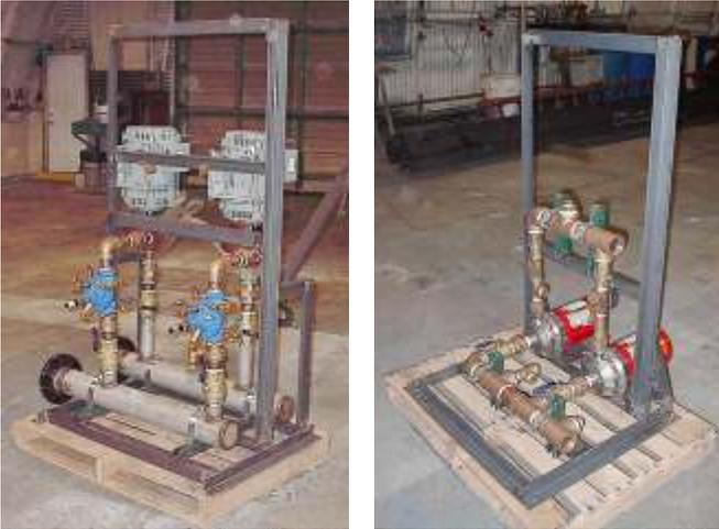
**Two Small Pump Skids** - Stainless steel frames, stainless and copper piping with valves from TriStar
