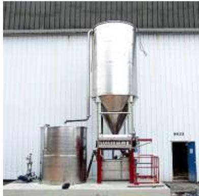
**Clarifier and Filter Press Skid** - New and refurbished components
