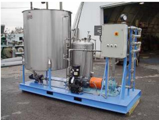
**Biodiesel Skid** - Fabricated for a biodiesel system OEM. Features new control panel, refurbished tank, and special mixing system.
