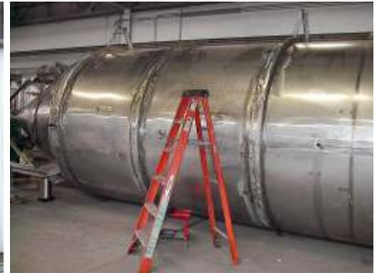
**Large Circular Clarifier** - Part of a larger filtration system, features all stainless tank and internal baffles
