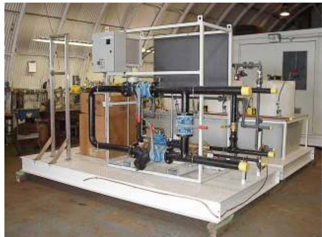
**Water Treatment System** - Complete package water treatment system including all piping, valves, pumps, controls, and enclosure
