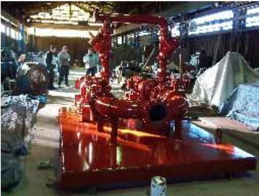
**Cooling Tower Pump Skid** - Dual pumps, basket strainer, common piping headers
