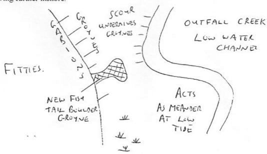
2. In the central promenade section between the Pier and Brighton slipway the groynes have proved to be ineffective. Here the beach in non existent and at high tide the waves directly attack the sea wall. The sea wall is beyond its design life and to extend its life and prevent further damage it is proposed to build a fish tail groyne of rocks and boulders. The aims would be threefold:-
