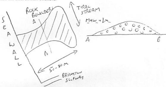
3. At Wonderland the wooden terminal groyne which is essential to the whole defence plan is in a very poor condition. Tidal scour and refraction around the end of the groyne are undermining the groyne and the southern end of the sea wall. It is proposed to build a new end to the groyne armouring it with stones and boulders, this should extend its life and prevent scour.
