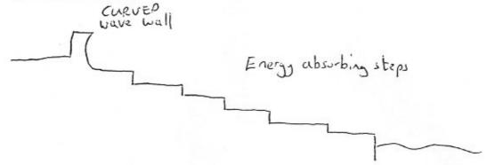
A. In the north is a stepped sea wall surmounted by a curved wave wall ( the curve reflects waves ) added in 1978.
