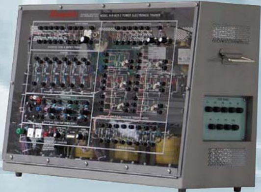
H-R-SCR-2 Power Electronics System
