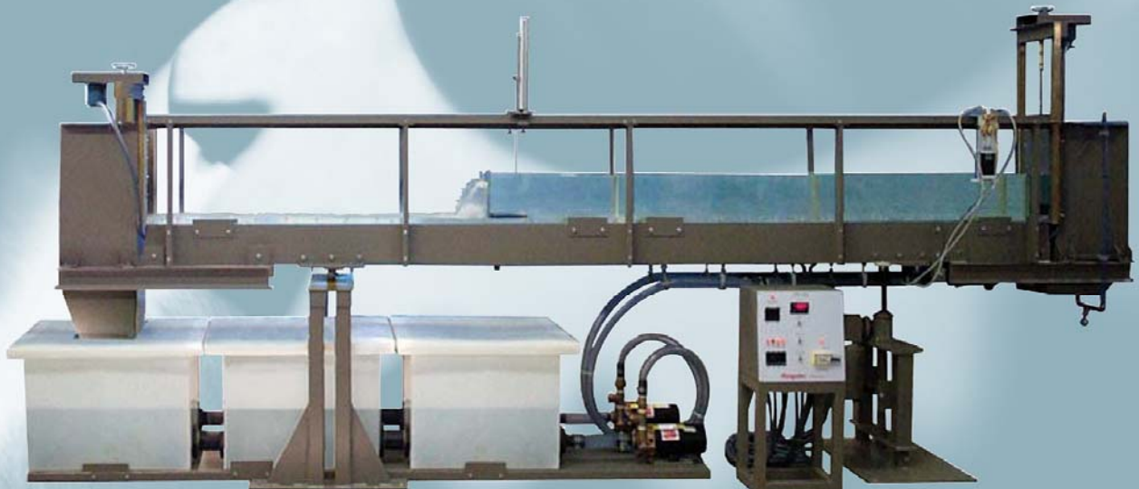
H-6531 Hydraulic Demonstration Channel
