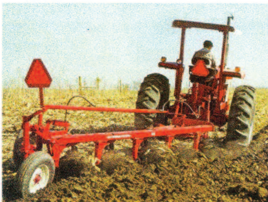
IH 1066 open station tractor with seat mounted SMV emblem. Plow has SMV emblem too.
