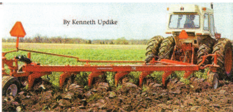
H 1466 w/ plow showing cab & plow mounting of SMV emblems.
