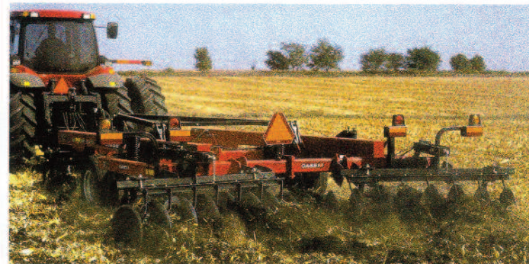
MAGNUM Tractor with 690 disc ripper showing SMV mounting and the wide extremity marker lighting.
