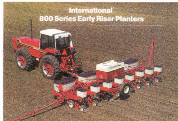
IH 3388 2+2 & IH 800 planter showing SMV mounting locations. The planter has 2 SMV's as it is an end tow unit.
