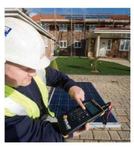
PV installation test IEC 62446 describes a variety of techniques for shorting a string during testing and taking measurements using clip-on ammeters.
