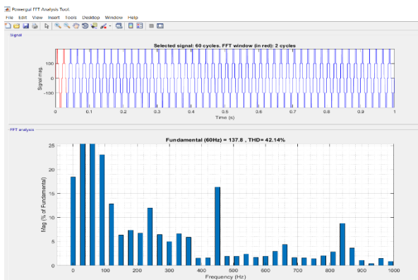
Figure 10: THD for Solar based Seven Level Inverter using Fuzzy Logic
