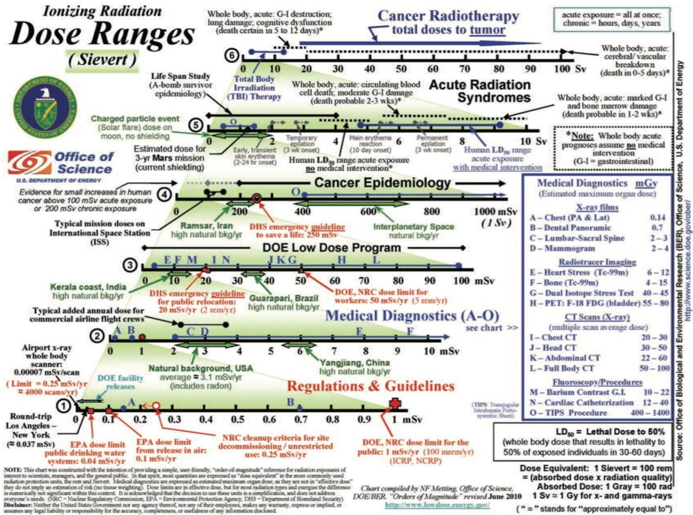
**FIGURE 17.4** This chart compiled by Dr.Noelle Metting, Office of Science of the U.S. Department of Energy, puts into perspective the different dose ranges relevant to radiation therapy, diagnostic radiology, and background radiation.
