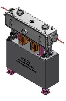
Additionally, the mirror can be positioned within the vacuum chamber through the use of ADC's 300 series precision jacks and slides. This series utilizes NEMA 23 stepper motors with Renishaw encoders to achieve great accuracy and repeatability. These are arranged in a way to provide 5 axis of movement to position the mirror.
