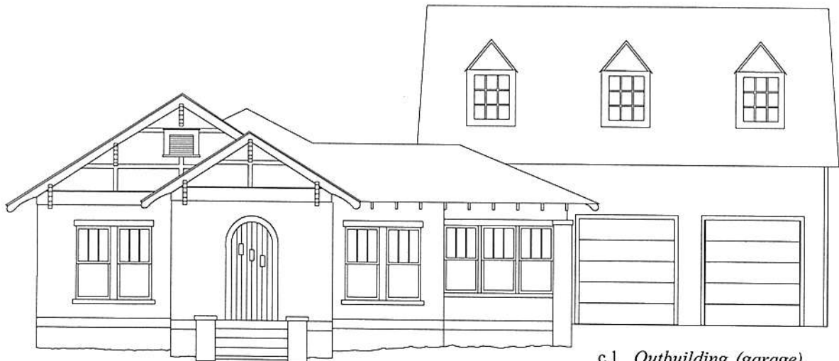
c.1 Outbuilding (garage) inappropriately scaled for the house
