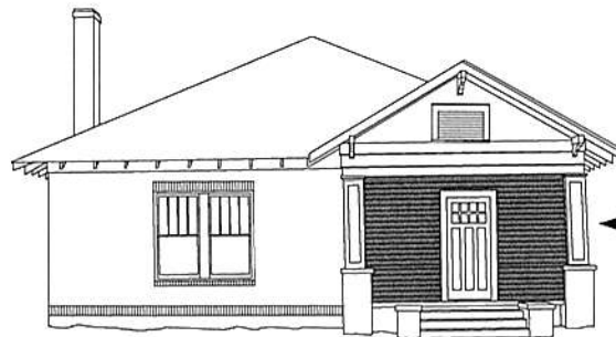
a.1 Inappropriate porch enclosure
