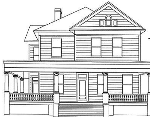
c.1 Inappropriate change in siding
