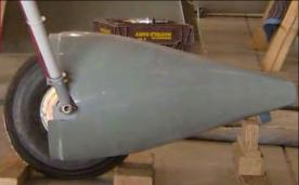
Note: A variety of different wood pieces are very helpful when fitting the wheel pants as the help to position the correctly while fitting.
