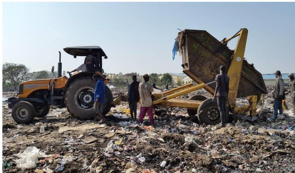
***Plate 16: Recommended skip system for expansion with some minor modifications***
