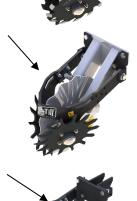
Properly designed row cleaners provide a very desirable type of tillage. With row cleaner teeth continuously engage the soil to the shallow depth of 1" to 1 1/2". By scarifying the soil's surface layer it makes it easier for the seed openers to open a well defined "V" without furrowing out or causing slabbing or fleaking. Eliminating furrows is the key to preventing erosion in the row on slopes and the ponding of water over the row in level areas. Martin Row Cleaners come in two basic
