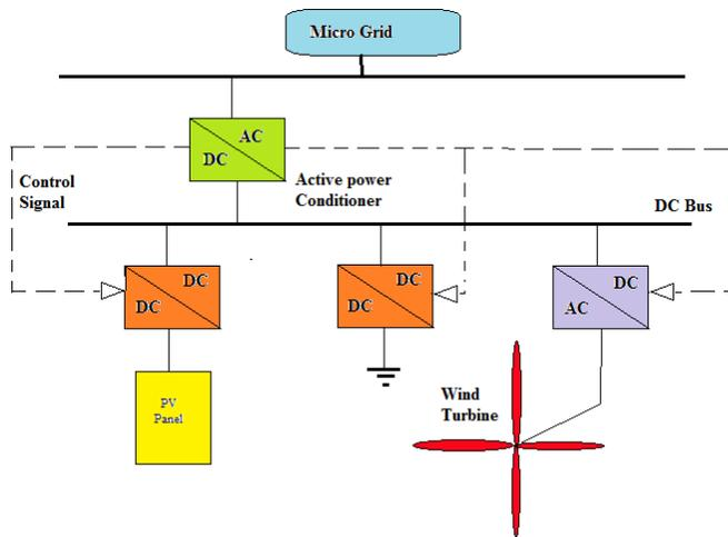
Figure 1. APC for Microgrid applications
