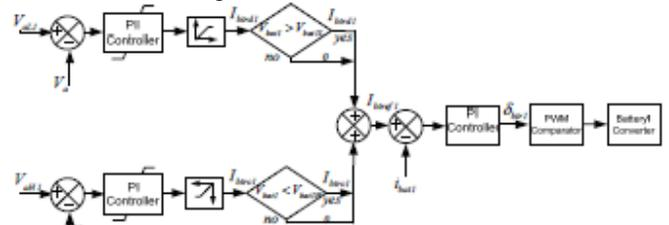
Fig. 5. Control loop of battery in ADCMG1.
