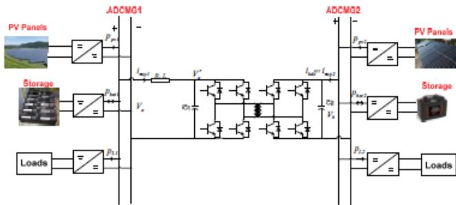
Figure 3: System architecture for interconnection of two ADCMGs.
