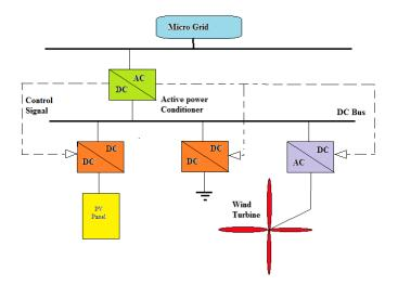
Figure 1. APC for Microgrid applications
