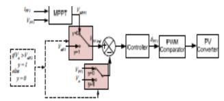
Fig. 4. Control loop of PV source in ADCMG1.
