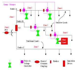
Fig.2 Microgrid Architecture
