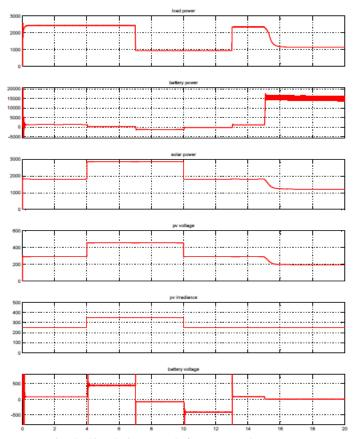
Fig. 8. Simulation Result for proposed system
