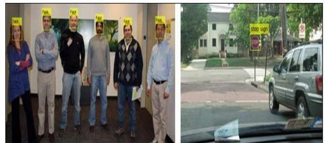
Fig 2: Face detection (left) and stop sign detection (right) using the Viola-Jones Object Detector.
