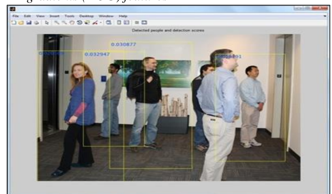
Fig 3: Human detection using pertained SVM with HOG features.
