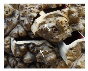
Before inserting the top-center drawer, first be sure that all drawers below it are installed. Slide in the top-center drawer until is stops with a click. This "click" is the locking pin from underlying drawers dropping. Now, pull gently on the middle-center drawer, and maintain this tension as the top drawer is pushed in. Pulling on the middle-center drawer temporarily restricts its locking pin from lifting back up, so the drawer above can be pushed fully back in.
