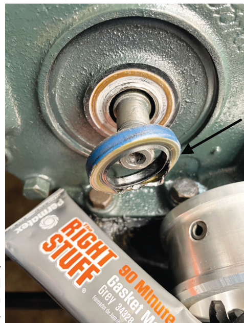
New modern seal in place with gray sealant. The seal that was removed showed a thin layer of blue silicone on a portion of the seal side surfaces.
