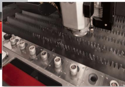
The FOL-AJ's high-speed shuttle tables and automatic nozzle changer maximize productivity. The shuttle tables externalize the material setup eliminating interference with the cutting process. The 8-station changer automatically changes, cleans and calibrates the nozzle based on material processing requirements (ensuring that the laser does not sit idle while waiting for an operator to set-up for the next job).
