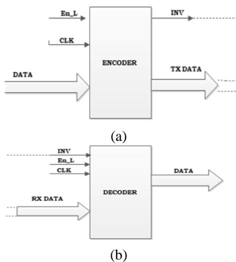
Fig.1 (a) Encoder (b) Decoder
