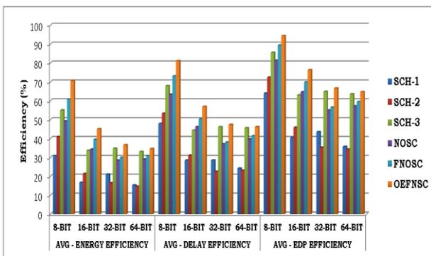
Fig.4: Energy, Delay, and Energy-Delay-Product (EDP) efficiency of data encoding techniques for 8-bit, 16-bit, 32-bit and 64-bit
