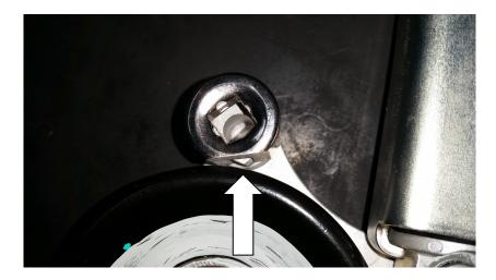
8) Torque socket cap bolts on pulley to 106 in.lb. Torque bolt on new idler to 33 ft.lb.
