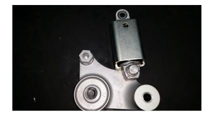
5) Now install KP oversize idler pulley and hand tighten nut for now.
