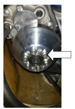
2) Using OE Spring Retaining Bracket, compress the spring enough to slide the bracket on. Remove tension, this will remove tension off your belt. NOTE: Not using this bracket can permanently damage your tensioner! If you need one, please contact us for ordering.
