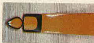
Close up view of the Fiberglass overlays on the bow tip.
