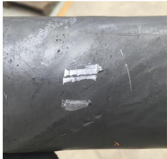
*Example of a scratched lead pipes showing shiny surface underneath.<sup>2</sup>*
