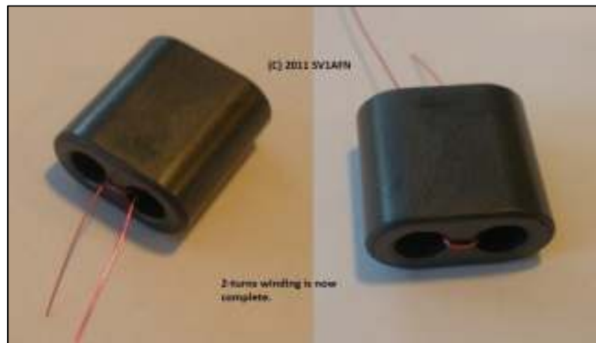
Photo 3. The completed 2-turn winding.
