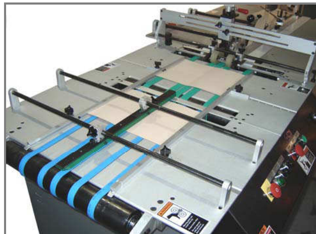
Product enters the KR 219 RSF and is side registered for consistent folding.
