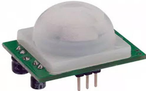
Fig.2: PIR(Passive Infra-red) Motion Sensor 6
